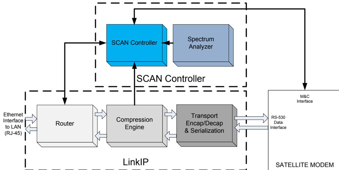
SCAN / LinkIP Functional Block Diagram
